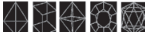
Figure. 6 Regular polyhedron: a . tetrahedron; b. hexahedron; c. octahedron; d. dodecahedron; e. icosahedron
